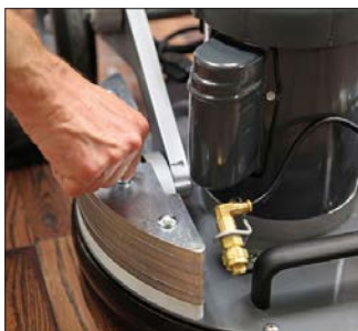
40 lbs of weight can be easily added for more down pressure.
